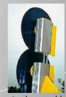
Thanks to a simple assembly design it is easy to add or remove additional cutting modules enabling you to turn 4 blades into 5 or 4 blades into 6, and so on.
