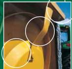
Replaceable skid shoes help protect the mower from damaging ground contact.
